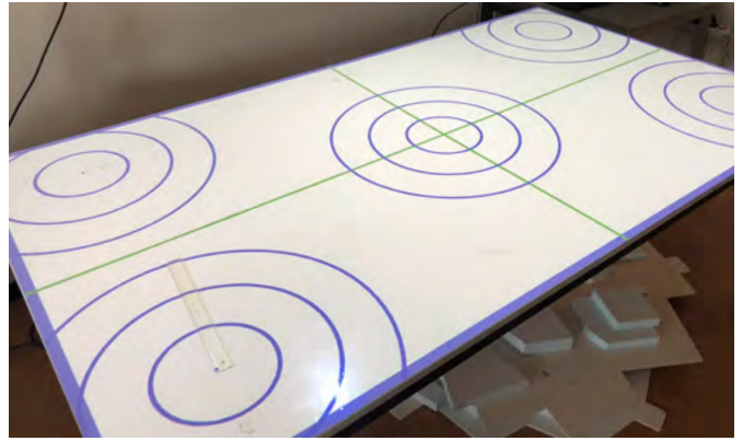
Fig. 2. Result of calibrating the projector.
