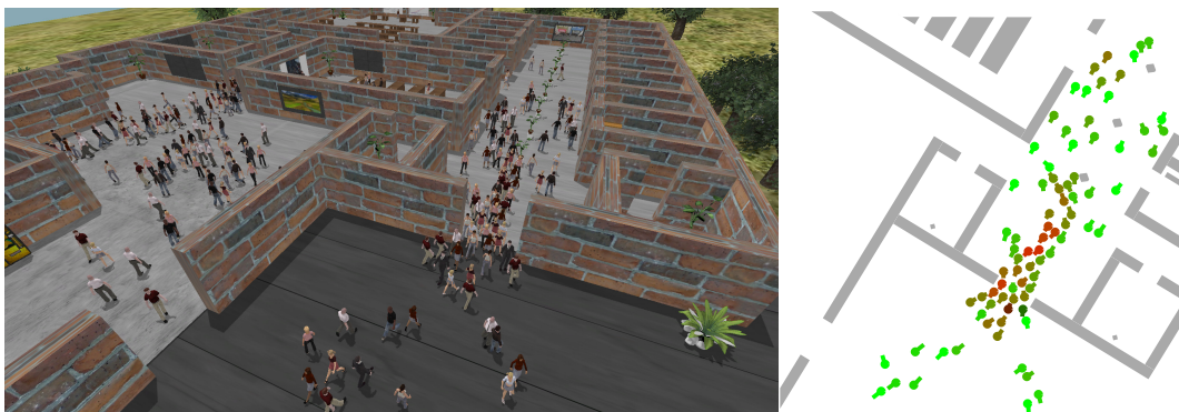
Figure 1: Left : A dense crowd of agents collaboratively moves through a narrow doorway. Right : A 2D representation of the doorway shows that each agent interpolates between individual behavior (green) and coordinated behavior (red).
