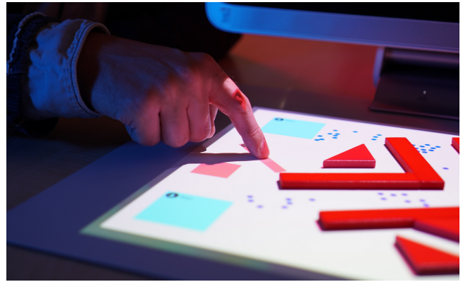
Figure 2: HP Sprout interface with blocks to build the environment and place start and target points for the crowd simulation.
