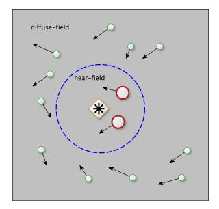
**Fig. 1:** Two acoustic regions are considered: diffusefield and near-field. Sound sources are individually spatialized (distance and position) in the near-field region only.
