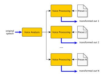
**Fig. 2:** Transformation presets can be generated automatically, producing several transformation files from a single speech input.
