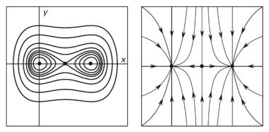
Figure: The level sets and phase portrait for the gradient system determined by  $V(x, y) = x^2(x-1)^2 + y^2$ .
