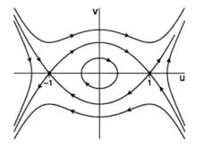
Figure: The phase plane of (1) in the (u, v) = (u, u')-plane.
