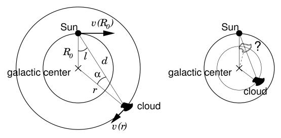
Figure 9: Geometry in measuring Dopplershifts of galactic clouds. Left: definition of various quantities. Right: knowledge of *l* and *r* leaves ambiguity in the location of clouds that orbit within the solar orbit.
