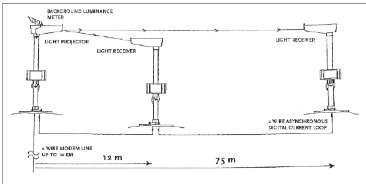
**Fig. 8.** A schematic of the transmissometer set up. The light projector and background luminance meter can be seen left, and both light receivers in the center and right side. Source: *KNMI (2005)*
