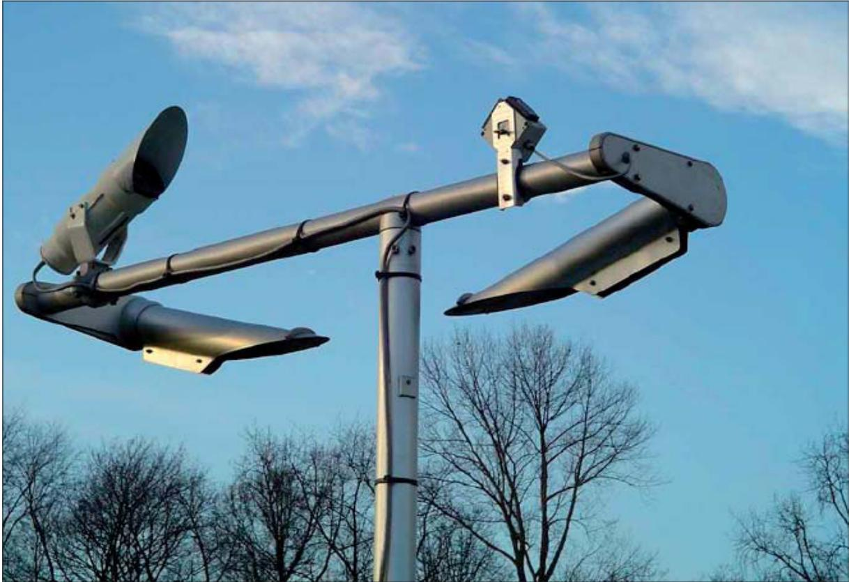
**Fig. 11.** A close up of the scatterometer, including a background luminance meter (left, pointing slightly upward) at de Bilt. Note the precipitation detector in the right side of the image. Source: KNMI (2005).
