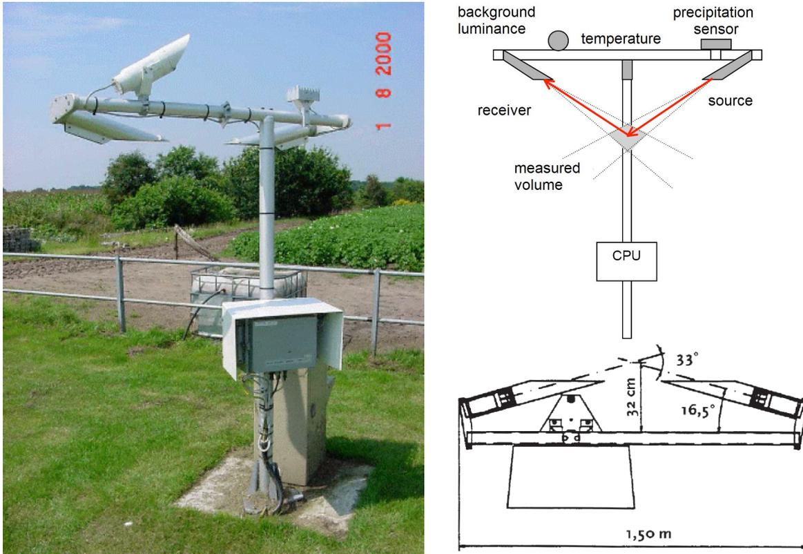
**Fig. 10.** The Vaisala FD12P present weather sensor (including scatterometer) and a schematic drawing of its most important features. Source: *KNMI, (2001)*: left & upper right (adapted); *KNMI (2005)*: below, right.
