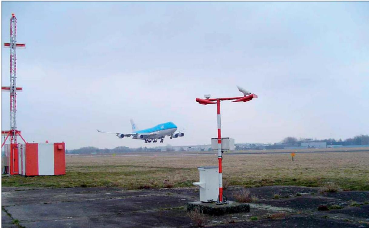
Fig. 12. A scatterometer with a background luminance meter at Beek, The Netherlands. Source: KNMI, 2005.
