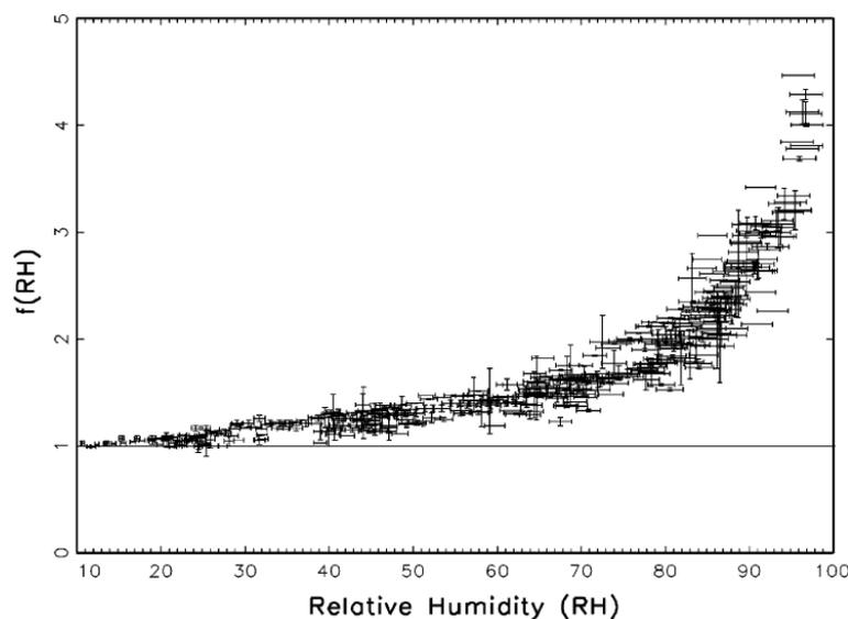
as a function of relative humidity  $f(\text{RH})$  of aerosols in the Great Smoky mountains. Note the rapid increase of scattering when RH becomes larger than 80%. This indicates that visibility will likely be much more sensitive to relative humidity changes when relative humidity is high, than when it is low.
