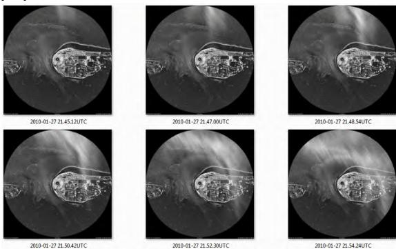
The figure above shows a series of radar images for a radar situated on top of the Ameland lighthouse on which a rainfall event can be seen. It is clear that in order to estimate rainfall from these images, a significant amount of filtering should be performed.
