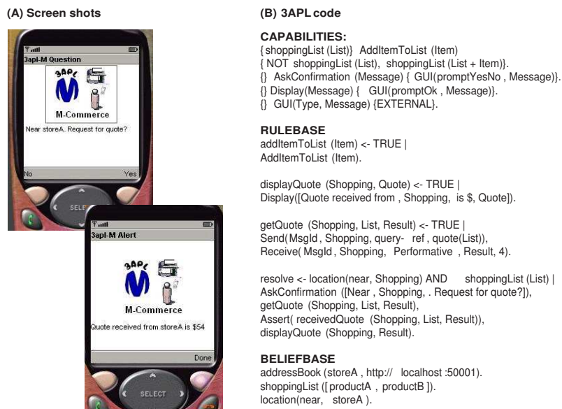
Fig. 7. Mobile Commerce Solution: (A) Conceptual Model and (B) 3APL code
