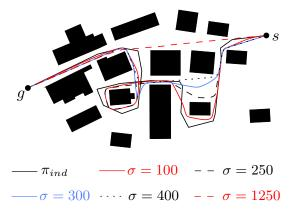
Figure 7: Output paths for different values of  $\sigma$ . The sampling distance d used in all examples is 20.
