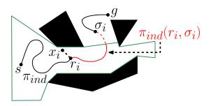
Figure 3: Visible parts of the environment and the indicative route from the current position  $x_i$ .
