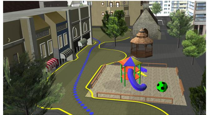
Fig. 1. A smooth, short path with clearance inside an Explicit Corridor.
