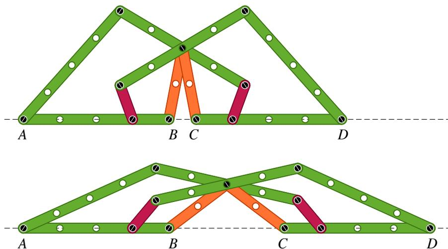
Figure 23: Kempe's sledge. If points  $A$  and  $B$  are kept fixed,  $C$  and  $D$  can only move on the dotted line. The four kite figures are all congruent.
