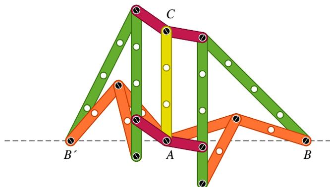
Figure 21: Kempe's construction leading to a straightedge.
