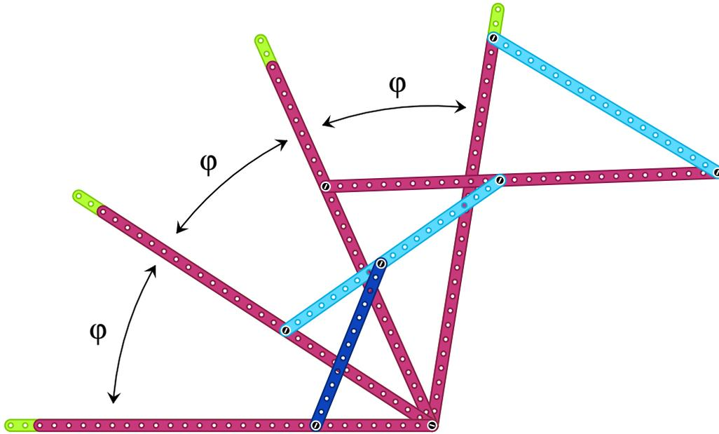
Figure 20: Kempe's trisector. The angles  $\varphi$  are the same. One easily sees how it works: a butterfly structure containing equal triangles is repeated twice, scaled down by a given factor (here  $2 : 3$ ). The basic strips have lengths 27, 18, 12 and 8.
