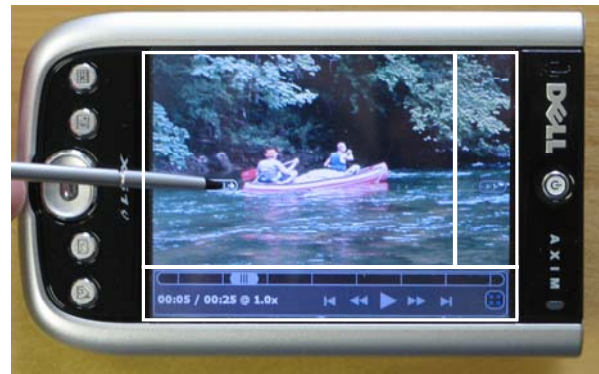
Figure 9. Regions for different kinds of interaction with the player software: Position-based navigation (top left), speed-based navigation (top right), and standard player widgets (bottom).
