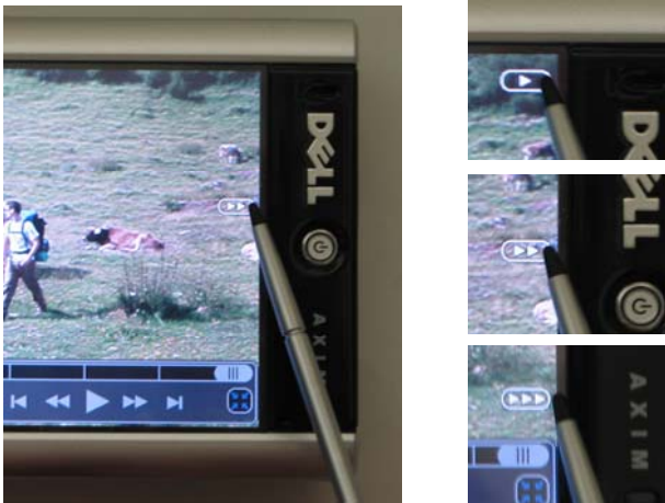
Figure 5. Speed-based skimming at the player's right border illustrated with different icons for different replay speeds.
