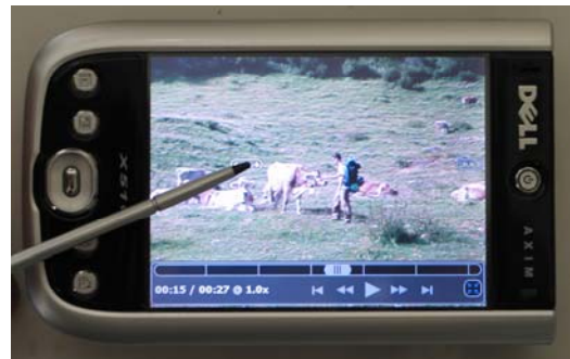
Figure 4. Full screen mode. The task bar with play/pause button, progress bar, etc. is faded in as soon as a user clicks anywhere on the screen and automatically disappears a few seconds after the user lifts the pen.
