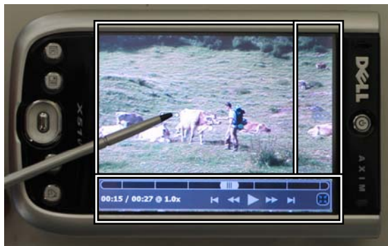
Figure 7. Illustration of regions with different functionality: Speed-based navigation (right), standard GUI components (bottom), position-based navigation (whole rest of the available screen space).
