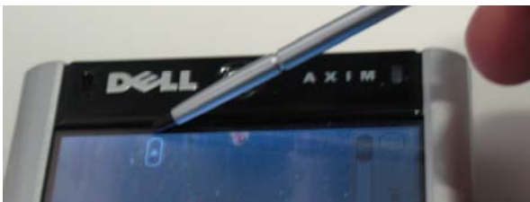
Figure 6. The physical border resulting from the slightly elevated case around the PDA's screen makes sliding of the pen at the right window border easy and comfortable.
