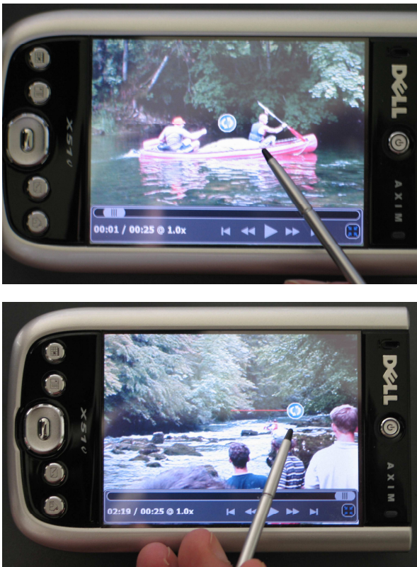
Figure 12. ScrollWheel: implementation on a PDA. (Top: position-based navigation via circular pen-movements around the screen's center. Bottom: speed-based navigation via horizontal pen-movements after grabbing the icon.)
