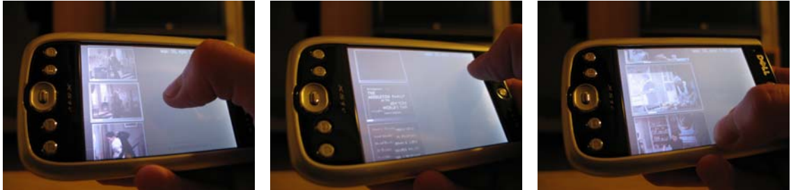
Figure 8. Different interactions with the implementation on a Dell Axim™ PDA: position (left), speed (right), and thumbnail size manipulation
