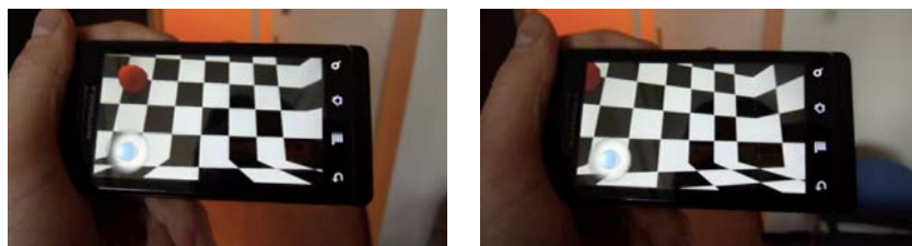
Fixed world approach (notice that the red sphere stays at roughly the same position with respect to the real environment; slight changes in position are due to sensor noise and the bigger field of view of the scene)
