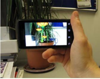
**Fig. 1.** Mobile Augmented Reality enhances reality (represented by the live video stream on your mobile) with 3D virtual objects (superimposed at a position in the video that corresponds to a related spot in the real world). In this example, a virtual flower grows in the real plant pot.
