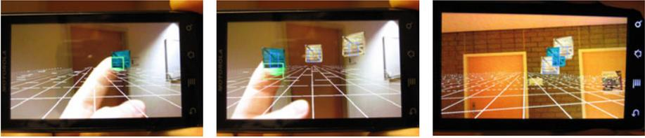
**Fig. 7.** Object selection task: test case (single object, left), easy (multiple non-overlapping objects, center), and hard (multiple overlapping objects, right)
