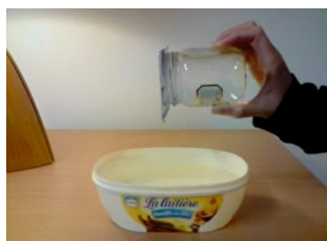
Figure 4 – Also in a horizontal position, the water does not flow out of the glass.
