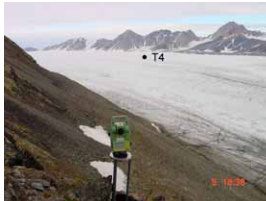
Figure 2. Electronic distance meter on a permanent metal tripod on the slope of Fugleberget. Location of stake T4 is marked on the Hansbreen surface (Photo by D. Puczko).
