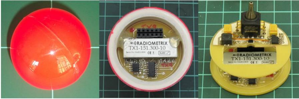
Figure 2. An electronic tracer (E-Tracer) for subglacial pressure sensing. The sensor package incorporates a radio chip which emits a signal to allow retrieval once the sensor has passed through the subglacial drainage system. The white potting mixture means that the sensor is neutrally buoyant, and the spherical shape allows it to pass through tortuous drainage conduits. The bright colour aids retrieval from the proglacial stream.
