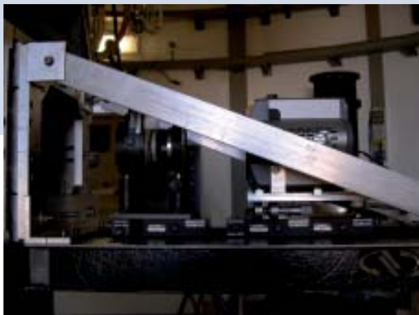
Image 1. FastCam prototype installed at the Carlos Sánchez telescope during one of the testing periods.
