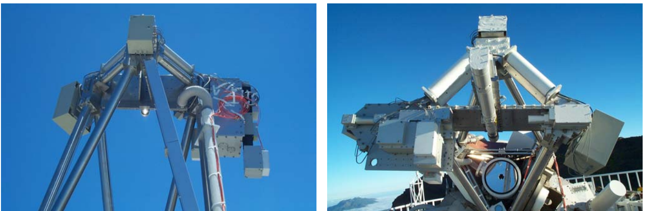
Fig. 3: Multi-wavelength system on the top of the telescope structure. The left image shows the water cooled diaphragm in the center of the picture. The front surface of the diaphragm is a mirror which reflects already most of the light. Only a field of 1.6mm diameter is used through a hole in the diaphragm. The primary solar image of 18.5mm diameter on the mirror is visible in the picture. After the diaphragm the light is guided to the multi-wavelength system visible at the right. Also visible at the right the hose for additional air suction around the diaphragm. Inside the hose are the invisible 2 small hoses for the water circulation through the diaphragm. The right image shows a top view of the upper part of the telescope structure. Visible are: to the left the multi-wavelength system, the primary mirror in the bottom center, the focus camera at the right and at the very right the box with control electronics. Below the primary mirror the entrance of the guider telescope is just visible.
