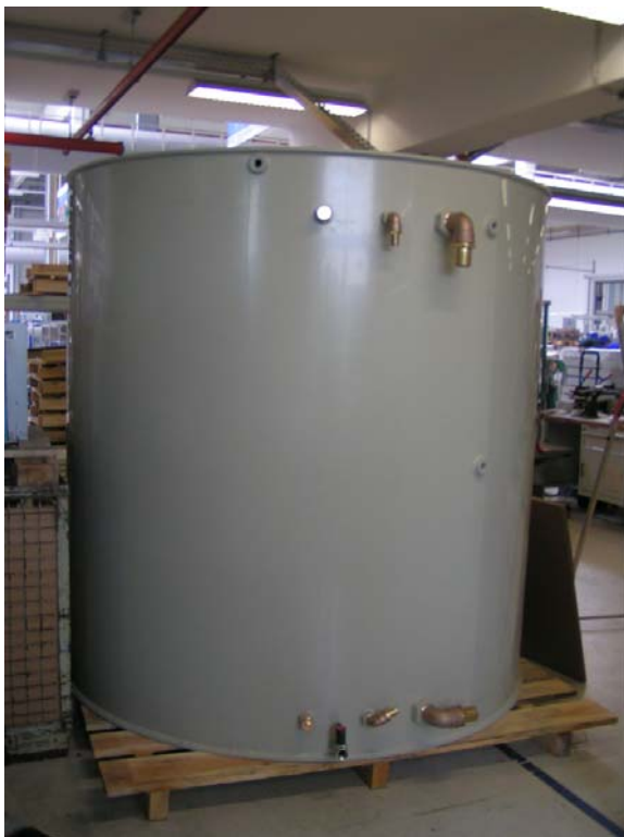
Fig. 9 Left: plastic watertank of 5 cubicm for heat storage. Right: radiator with fan for fast heat release only during sunrise and sunset.
