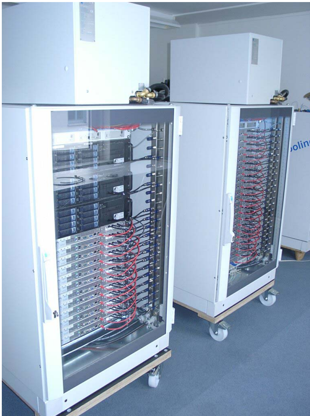
Fig. 7: The 2 racks with the 70 processors on 35 boards and the 15 hard disks of each 300GB divided over 3 units with a board and 5 harddisks each in the upper part of the rack to the left. To each board are two cables and two waterhoses. From left to right are visible for each board the following connections:
