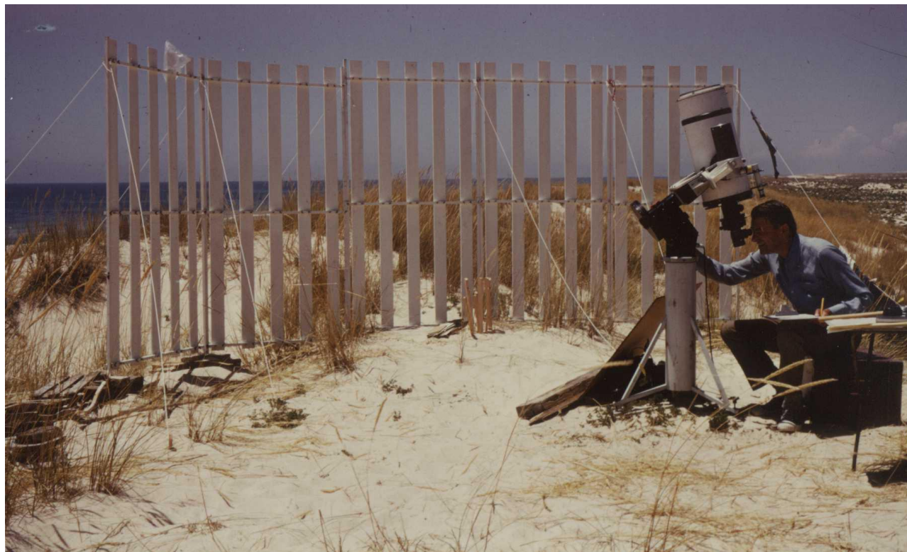
Fig. 7. Kees Zwaan doing site testing with a commercial 20-cm Maksutow telescope protected against wind shaking by a semitransparent windshield on top of a sand dune on a lagoon island at the south coast of Portugal.
