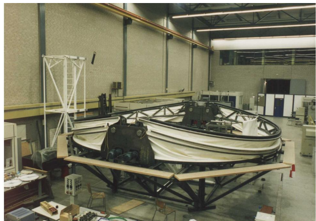
Fig. 1. Test assembly of DOT-tent at the workshop in Delft. Left : tent closed; Right : tent open.
