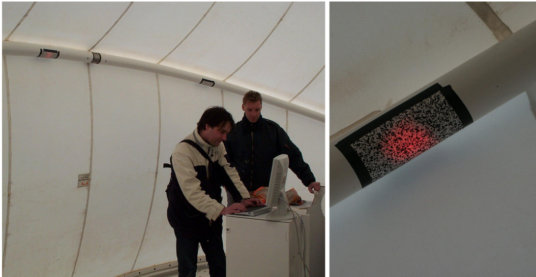
Fig. 6. Left: Measuring activity on the platform. 2 target points on a bow are visible. Right: Close-up of target point with light spot.
