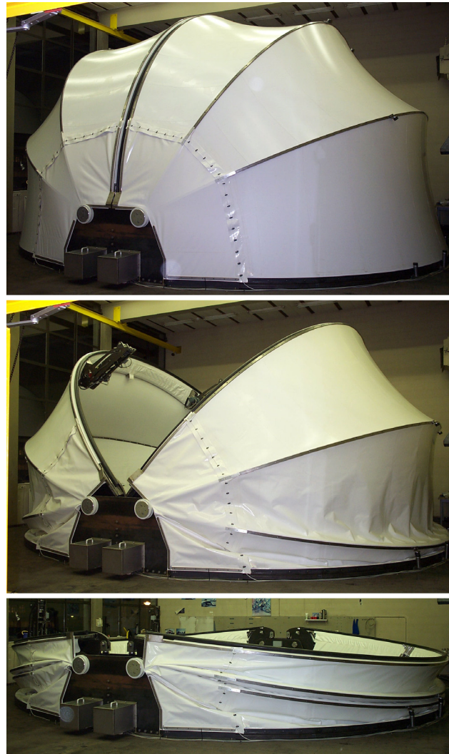
Fig. 8 The GREGOR dome in the assembling hall of the workshop DEMO at Delft. Top: closed. Center: half open. One of the clamps is well visible, the second one is for a large part hidden behind the dome segments in front. The clamps divide the main bow in about three equal parts of 60°. Bottom: open.
