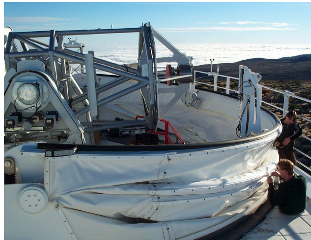
Fig. 16 Sensors on and around the GREGOR dome. The pressure sensors on the bows were just mounted. The wind cups and vanes were already mounted on the fence around the platform for some time. There are nine sets of which three are visible in the picture.
