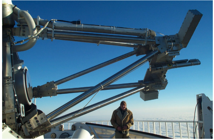
Figure 13: The open structure of the DOT telescope. To the left the primary mirror, to the right the secondary optics (in the telescope top), which for the DOT includes a multi-channel system.
