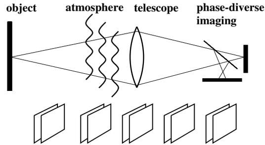
Figure 4: Phase-diverse speckle image registration. Following an idea originally due to Högbom (in Rutten and Severino 1989), synchronized short-duration (about 10 msec) pairs of granulation exposures are registered both in focus and out of focus. Five pairs suffice to produce reliable restoration of the wavefront to the telescope diffraction limit when the seeing is reasonable.
