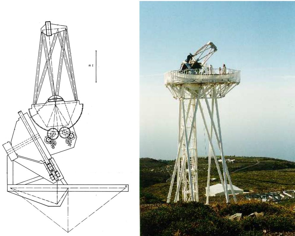
Figure 3: Left: sketch of the DOT pointing at the sun from La Palma at noon on June 21. The bar measures 1 m. Right: The DOT on its tower, La Palma, October 1996. North is to the right. The building of the Carlsberg transit telescope, HEGRA and the Residencia are seen in the background.
