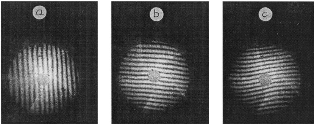
Fig. 2. Interferograms of the primary mirror. *a* and *b*: perpendicular interference fringes near the focus of the paraboloid. *c*: coma outside the region around the focal point of the paraboloid. The DOT field is small enough for no coma correction to be necessary.
