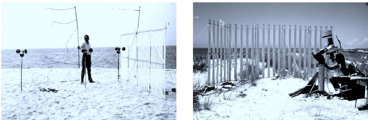
**Figure 2.** Zwaan site testing on Barreta. Left: demonstrating the effect of the semi-transparent wind screen. Right: monitoring solar image quality on the Kiepenheuer scale. From slides taken by R. Hammerschlag in 1973.
