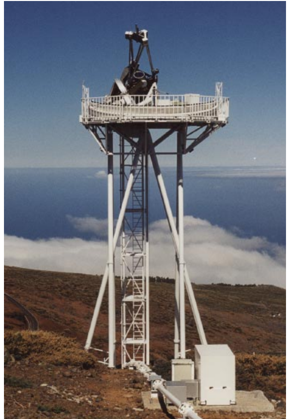
Figure 1: The Dutch Open Telescope on La Palma. The telescope and the 15 m high support tower are open to the trade wind from the North (to the right) which brings the best seeing to La Palma. When it blows sufficiently strong it confines the solar-heated boundary layer of turbulent convection to heights below the telescope and flushes the telescope itself. The parallactic telescope mount is extraordinarily stiff to avoid image shake from wind buffeting. A clamshell foldaway dome protects the telescope from (sometimes very) inclement weather. The telescope consists of a 45 cm parabolic primary (seen in the middle of the photograph) with 200 cm focal length. The primary image is mostly reflected away with a water-cooled mirror (the water storage tank is in the foreground). A small hole (1.6 mm) transmits the field of view. The slender on-axis pipe at the top of the telescope contains the focusing mechanism, re-imaging optics, the G-band filter and the G-band camera. The other four cameras of the multi-channel imaging system will be mounted at the telescope top besides the incoming beam. The speckle frames are transported by optical fibers (in the pipe) to a large-capacity data acquisition system in the Swedish solar telescope building from which the DOT is operated. Picture taken by Aswin Jägers.
