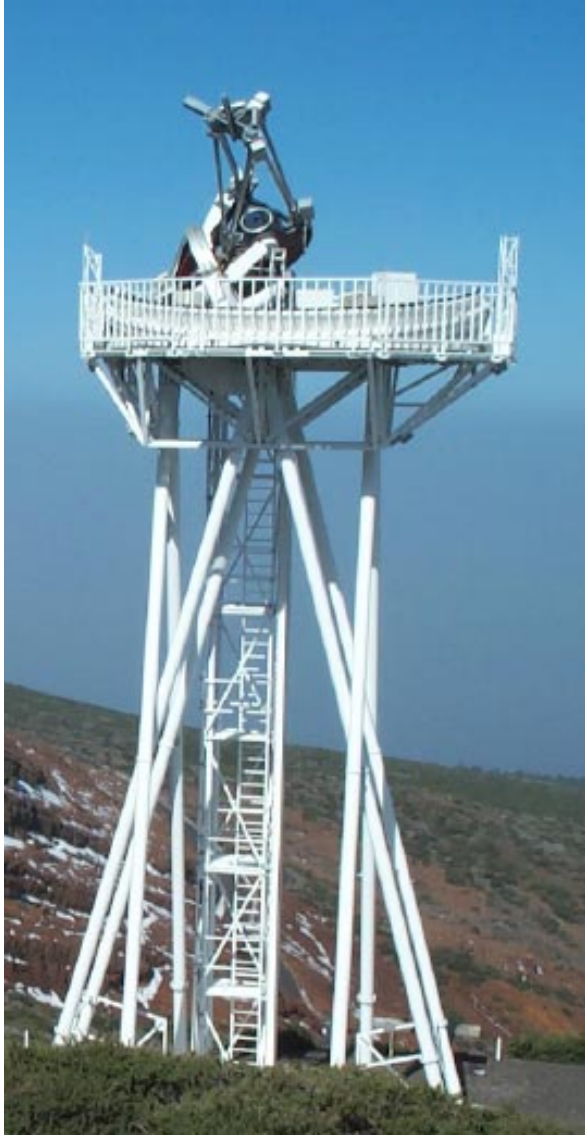
Figure 1: The Dutch Open Telescope at the Roque de los Muchachos Observatory. The 15m high tower as well as the telescope itself are open to the trade wind from the North (to the right). When it blows strongly it skims off the solar-heated turbulent boundary layer and flushes the telescope itself. The parallactic telescope mount is extraordinarily stiff to avoid image shake from wind buffeting. A clamshell foldaway dome protects the telescope from (sometimes very) inclement weather. The DOT presently has a 45 cm parabolic primary mirror with 200 cm focal length. The prime-focus image is mostly reflected away with a water-cooled mirror containing a 1.6 mm hole which transmits the field of view. The structure at the top of the telescope contains this light stop, the focusing mechanism, re-imaging optics, the G-band filter and the G-band camera in a slender on-axis tube, a phase-diverse video imaging system for focus control branched off on one side of the incoming beam, the near-G continuum filter and camera on the other side. The Ca II H\alpha and Ba II 4554 Å filters and cameras will be mounted there as well. The speckle frames from each camera are transported via optical fibers to the large-capacity (360 GByte) specklegram acquisition system in the DOT control room in the nearby New Swedish Solar Telescope (NSST) building.
