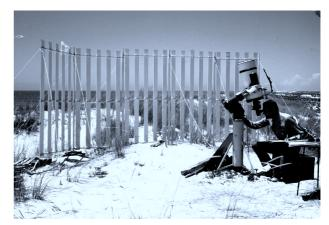
Figure 2. Zwaan site testing on Barreta. Left: demonstrating the effect of the semi-transparent wind screen. Right: monitoring solar image quality on the Kiepenheuer scale. From slides taken by R. Hammerschlag in 1973.
