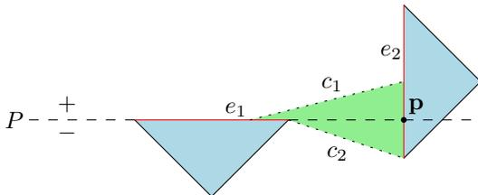
Fig. 4. Connection  $c_2$  has a vertex on the negative side of the associated plane  $P$  of  $e_1$ . We restrict that vertex of  $c_2$  to the intersection of  $P$  and  $e_2$ , represented by point  $\mathbf{p}$ . If no intersection exists, we detect no gap between the two edges.
