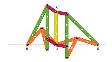
Figure 21: Kempe's construction leading to a straightedge.
