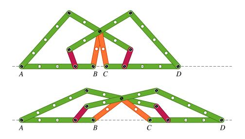
Figure 23: Kempe's sledge. If points A and B are kept fixed, C and D can only move on the dotted line. The four kite figures are all congruent.
