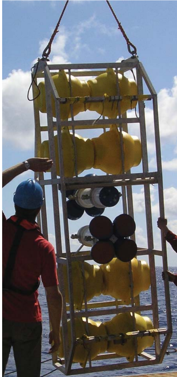
Figure 3. DTV with up- and down-looking ADCP's pulled sideways above deck.
