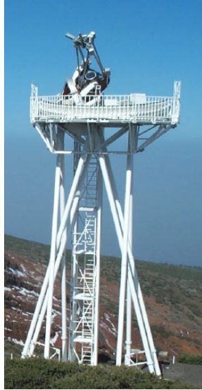
Figure 1: Left: Dutch Open Telescope on La Palma. The DOT is mounted on a 15-m high open tower to exploit the superior atmospheric seeing brought by the oceanic trade winds. The clamshell bad-weather canopy is folded away in this view. The 45-cm parabolic primary mirror is seen at the center of the telescope structure. The post-focus system is mounted at the telescope top. The digital image stream is transported through fibers to the control room in the nearby Swedish SST building. Right: optics diagram of the tomographic multi-wavelength system feeding six identical speckle cameras synchronously with speckle bursts in the blue continuum (432.0 nm, deep photosphere, granulation), red continuum (651.0 nm, linear Rayleigh-Jeans temperature sensitivity, wide-band reference for H\alpha restoration), G band (430.5 nm, molecular CH lines showing photospheric fluxtubes at enhanced contrast; this channel is mounted separately in the on-axis tube seen in the photograph), Ca II H (396.8 nm, low-chromosphere magnetism, well-suited for precise co-registration with ultraviolet images from space), H\alpha (656.3 nm, low-lying loops in magnetic canopies) and Ba II (455.4 nm, heavy-ion line optimally suited to Doppler and Hanle mapping). The latter two channels use large tunable Lyot filters.
