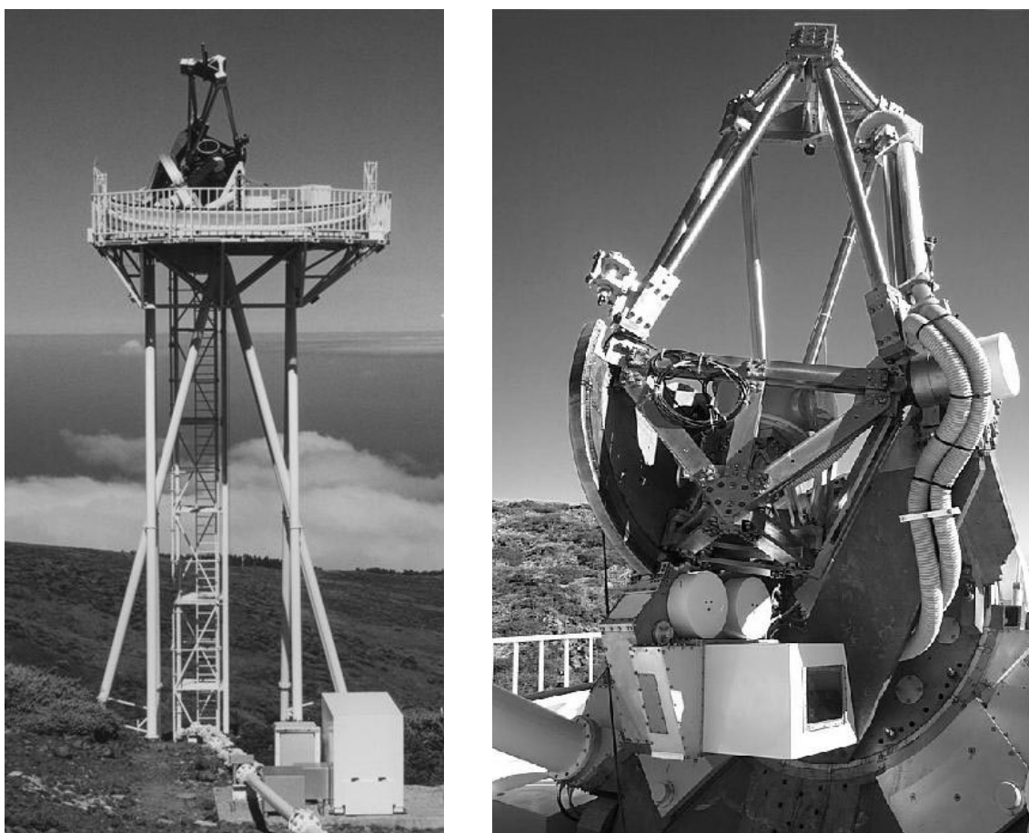
Figure 2: The Dutch Open Telescope (DOT) on La Palma. Left: telescope with 45 cm primary mirror and 15-m high support tower, both open to the strong trade winds that come in from the right (North). The inversion layer (ocean clouds) is well below the volcano rim (2400 m) during the summer. The clamshell bad-weather canopy is folded away but is needed in winter when the weather can be a killer combination of heavy fogs, ice deposition, and storms. The white box contains a water tank for prime-focus cooling. The pipe transports control commands and digital images from/to the control room in the nearby Swedish telescope building. Right: parallax telescope mount. The heavy construction and the extraordinary stiff gears avoid image shake from wind buffeting. The on-axis tube at the top contains a water-cooled tilted mirror which reflects the primary solar image away except for a 1.6 mm hole transmitting the 2 arcmin field of view to the focusing mechanism and re-imaging optics. The primary beam continues to the G-band filter and CCD camera. Four more cameras are being mounted along the telescope top besides the incoming beam. They are fed by beamsplitters and dichroic mirrors plus multi-wavelength re-imaging optics (continuum, Ca II K, H-alpha, Ba II 4554). The continuum channel became operational during the USO jubilee meeting and serves to separate granules and G-band bright points. The Ca II K channel will image the low chromosphere and permit exact co-alignment with TRACE sequences including near-ultraviolet imaging. The rationale to add H-alpha is given above; the DOT will use the tunable Zeiss filter formerly at Gaizauskas' ORSO. The Ba II 4554 Å line is a very promising Doppler diagnostic (Sütterlin et al. 2001b). More detail and photographs at http://dot.astro.uu.nl .
