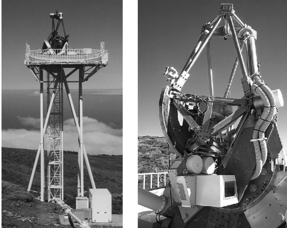
Figure 1.1. Hammerschlag's Dutch Open Telescope on La Palma. Left: telescope with 45 cm primary mirror and support tower, open to the trade wind from the North (to the right) which brings the best seeing. The inversion layer (clouds) is far below the 2400 m high volcano rim. The clamshell bad-weather canopy is folded away. The white box contains a water tank for prime-focus cooling. The pipe transports control commands and digital images from/to the control room in the Swedish telescope building. Right: the parallactic telescope mount is extraordinarily heavy and stiff to avoid image shake from wind buffeting. The slender on-axis pipe at the top contains a water-cooled tilted mirror which reflects the primary solar image away except for a 1.6 mm hole transmitting the 2 arcmin field of view to the focusing mechanism, re-imaging optics, G-band filter and CCD camera. More photographs at http://dot.astro.uu.nl .
