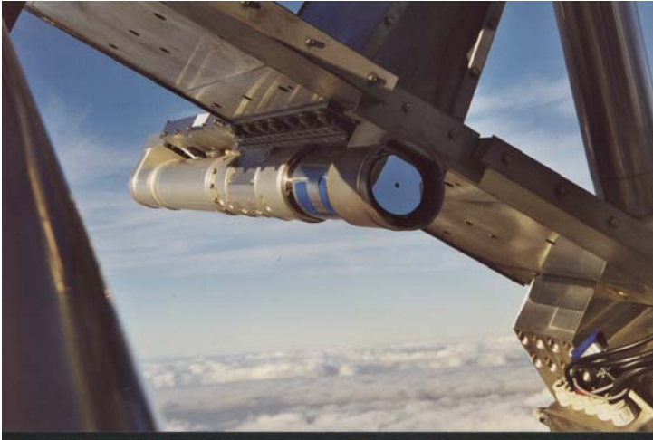
Fig. 5: Field stop mounted on the front side of the secondary optics. The surface is coated with protected silver. In the center the hole with 1.6 mm diameter is visible.
